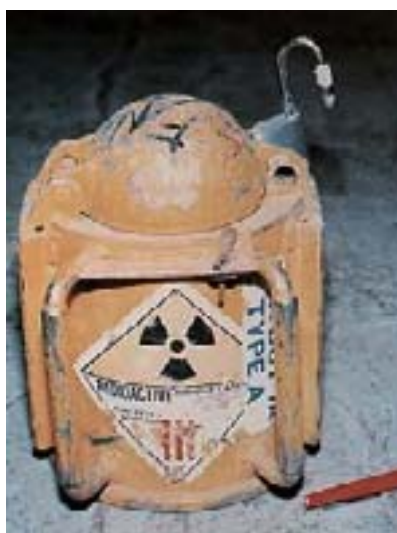
A transport container for radioactive materials recovered by the IAEA
