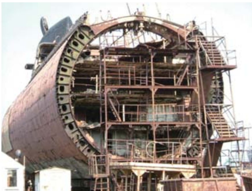
Dismantling of a submarine (Victor III-class decommissioned nuclear submarine) at the Zvezda Shipyard
