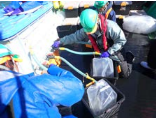
Collecting samples of surface seawater for H-3 analysis off the coast of TEPCO's Fukushima Daiichi Nuclear Power Station (October, Fukushima Prefecture; Photo: Nuclear Regulation Authority)
