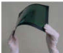
Thin-film perovskite solar cell (Photo: Toshiba Corporation) (Note) This achievement is the fruit of work commissioned by the New Energy and Industrial Technology Development Organization (NEDO).
