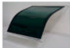
Thin-film perovskite solar cell (Photo: Toshiba Corporation) (Note) This achievement is the fruit of work commissioned by the New Energy and Industrial Technology Development Organization (NEDO).
