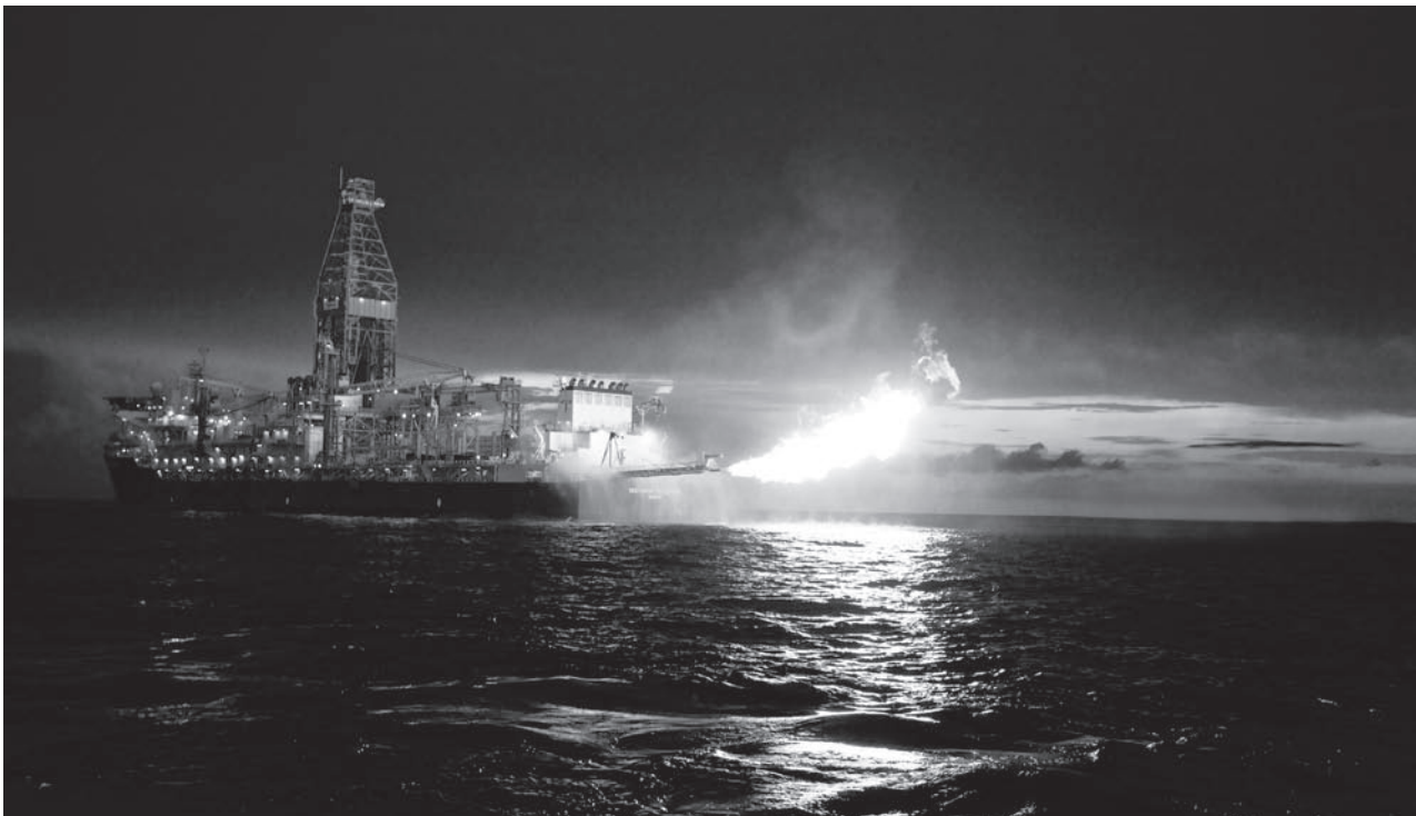
A drill ship conducting productivity tests at a gas field already discovered off the coast of Mozambique (a ship equipped with gas field exploration and drilling facility) (Photo: Anadarko Petroleum Corporation)
