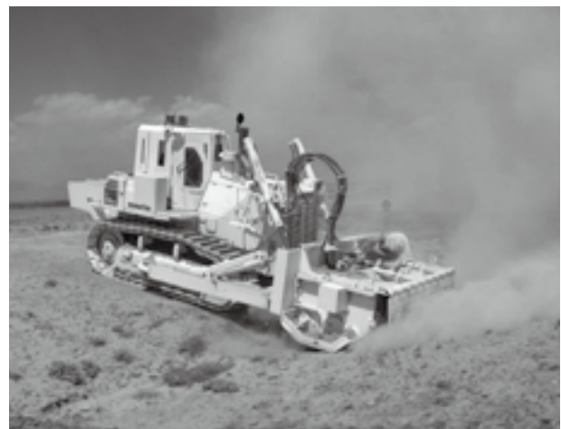
Antipersonnel landmine removal machine that was demonstration tested onsite in Afghanistan (Photo: Komatsu)
