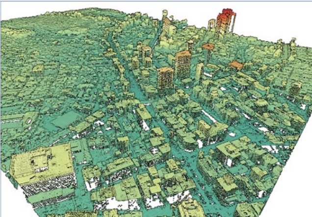
Highly precise elevation data (3D point cloud) (Photo: Geospatial Information Authority of Japan)
