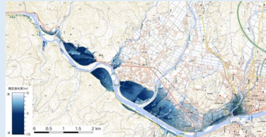
Estimating inundation depth from elevation data (Photo: Geospatial Information Authority of Japan)
