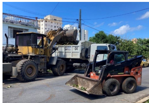
Disaster waste removal in progress: Dump truck and skid steer loader
