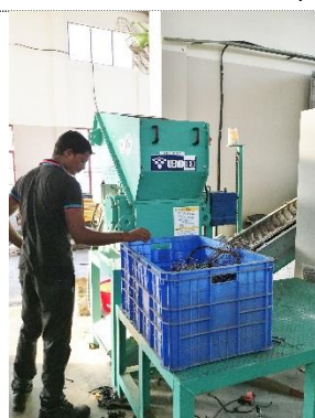
Extraction of copper from recycled automobile parts(Verification Survey with the Private Sector for Disseminating Japanese Technologies for the environmental and advanced recycling for copper resources of wire harness in the automotive dismantling recycling business)
