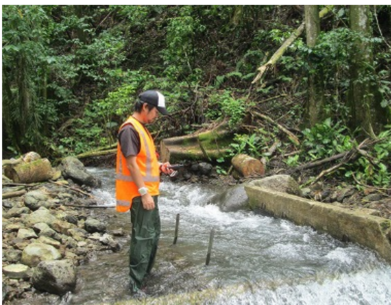
Measurement of the location of the sluice gate at Vailima intake by GPS
