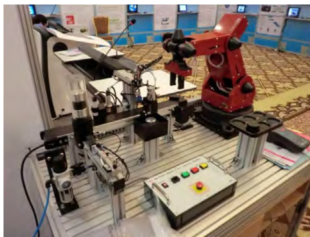
図 2-1 ROBOT & PLC CONTROL TRINER (ED-7255T) ED Corporation 製
