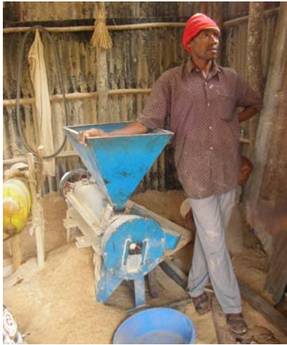
Figure 19a: Typical locally fabricated rice mills used in Uganda
