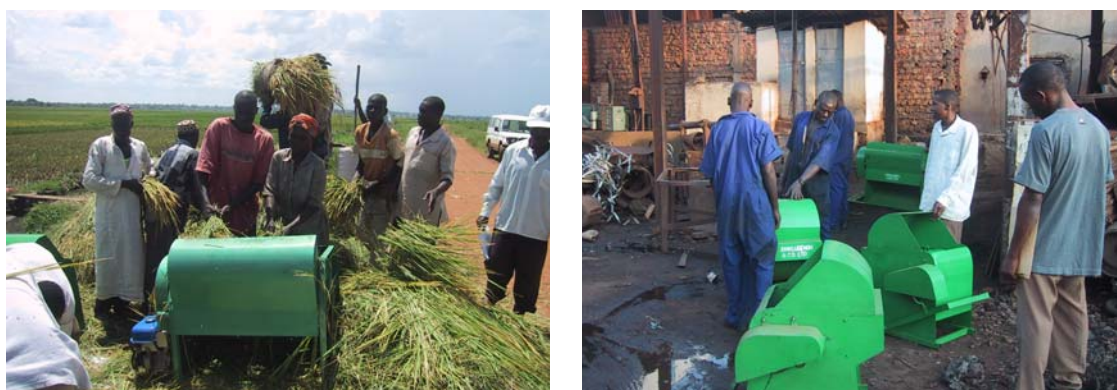
Figure 16: Field testing of rice thresher & rice equipment fabrication at NVTI
