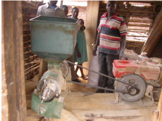
Figure 19a: Typical locally fabricated rice mills used in Uganda
