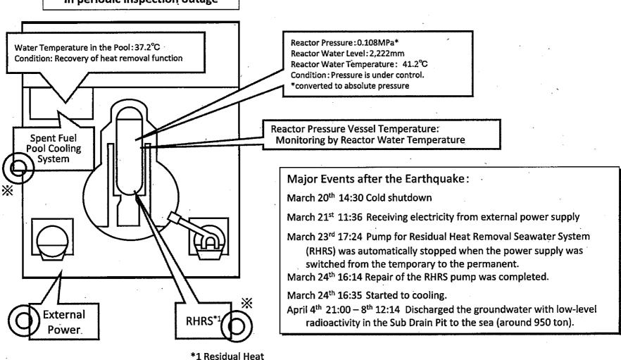
※Heat removal was carried out alternately with the water in the Reactor Core and in the Spent Fuel Pool.
