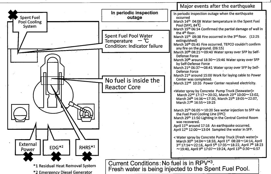
\*3 Reactor Pressure Vessel
