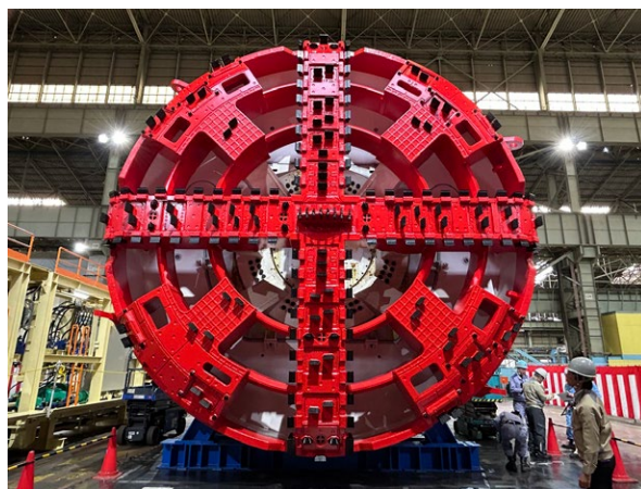
A tunnel boring machine used for excavation under the yen loan “Metro Manila Subway Project” (Photo: Sumitomo Mitsui Construction Co., Ltd.)
