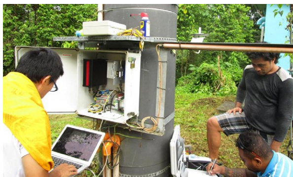
A JOCV engaging in activities such as maintaining meteorological observation equipment installed through Grants and delivering weather information using ICT (information and communications technology) at the Samoa Meteorology Division (Photo: JICA)
