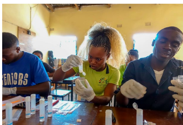
Coliform testing of samples collected by a youth group in Lusaka City under the "Project for Risk-based Participatory WASH Planning and Citizen-data WASH Statistics for African Peri-urban Settlements" (SATREPS) in Zambia (Photo: Hidenori Harada)
