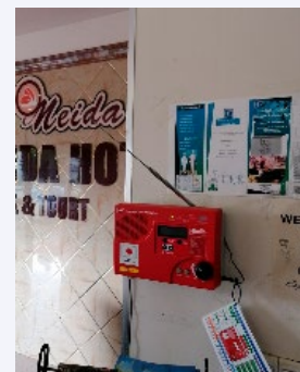
Remote Activated Receiver (RAR). An "indoor siren terminal" installed to expand and complement the range of siren alarms at approximately 500 locations nationwide. (Photo: The Consortium of Yachiyo Engineering Co., Ltd., Japan Telecommunications Engineering and Consulting Service, and Kokusai Kogyo Co., Ltd.)
