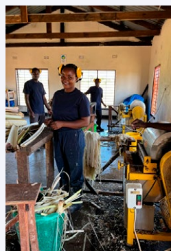
Local staff of the company operating a machine that extracts fibers from banana stems (Photo: JICA)
