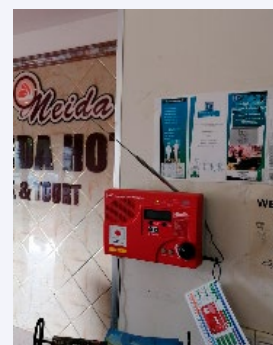
Remote Activated Receiver (RAR). An “indoor siren terminal” installed to expand and complement the range of siren alarms at approximately 500 locations nationwide. (Photo: The Consortium of Yachiyo Engineering Co., Ltd., Japan Telecommunications Engineering and Consulting Service, and Kokusai Kogyo Co., Ltd.)
