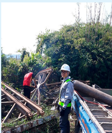
Dr. Thavone confirming the strength of the components of a collapsed Bailey bridge, as part of his research activities in Laos (Photo: Nagasaki University)
