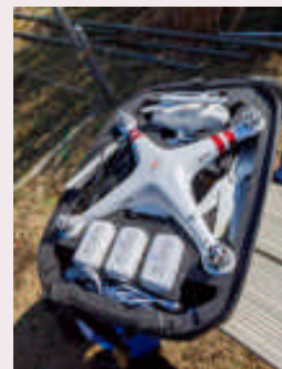
Drone used for demonstration experiment for the acquisition and analysis of thermal images of landmines and unexploded ordnance
