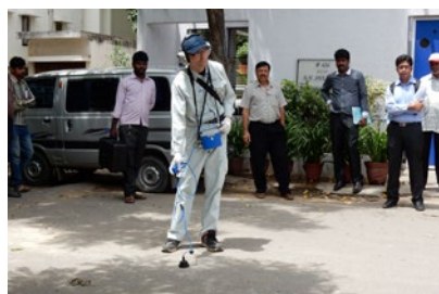
Technical training on water leakage detection using a leakage detector: the sound of water dripping is detected with a flashing LED light.
