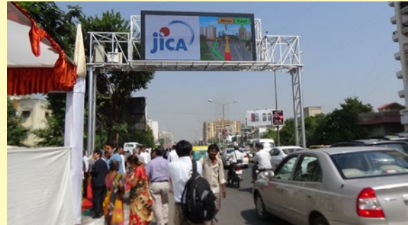
Traffic congestion information delivering system (Photo: ZERO-SUM LTD.)
