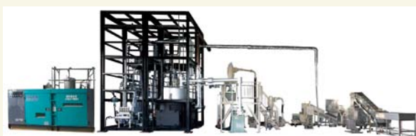
Composition of pre-treatment equipment and waste plastic-to-oil production system (Photo: CFP Corporation)
