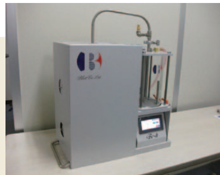
A desktop-type waste plastic-to-oil system. (Photo: Blest Co., Ltd.)
