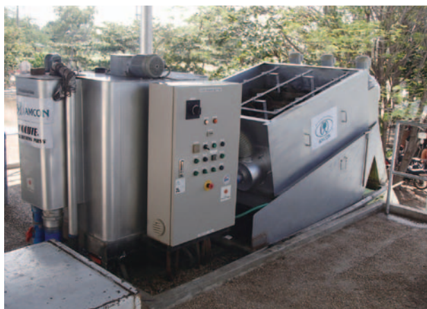
Dewatering equipment with sludge treatment capacity of 10t per hour. The equipment, which features power and water saving and ease of operational control enables unattended operation around the clock. (Photo: AMCON INC.)
