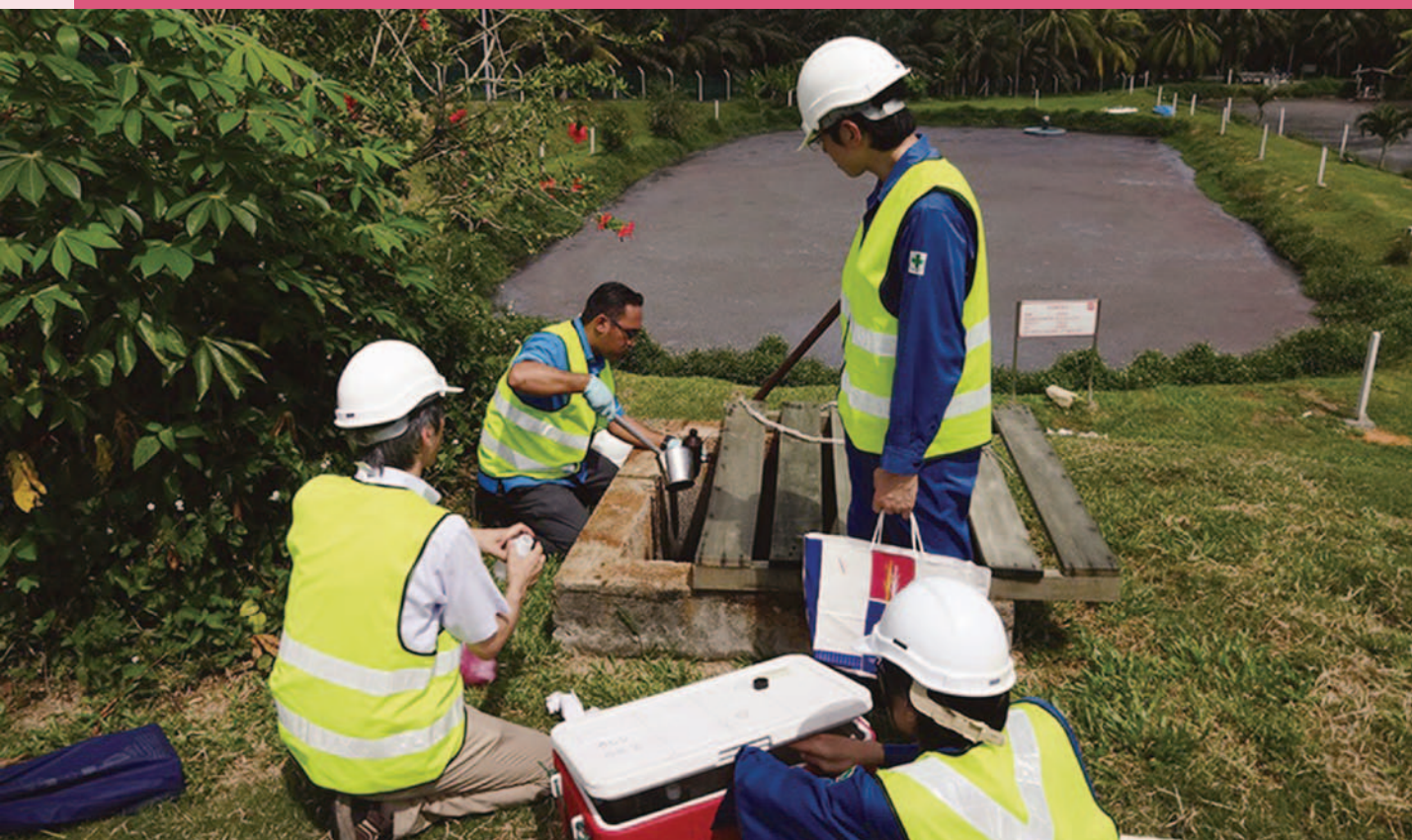
A Hanshin Engineering team collects water samples from an existing water treatment lagoon pond to survey water quality at a palm oil factory in Malaysia.
