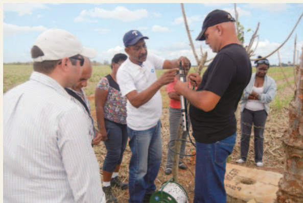
Engineers of EIPH-Habana receive training on methods for measurement of water quality at different depths of the measurement wells using multi-parameter water quality analyzers. (Photo: Hirokatsu Utagawa)
