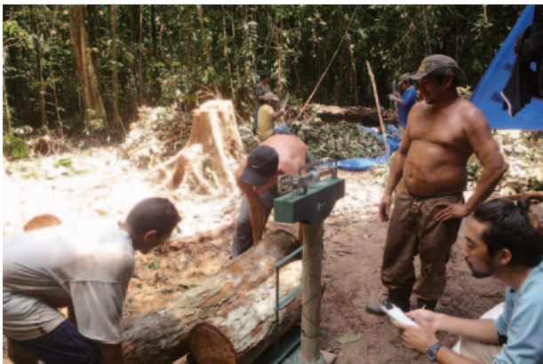
"Ground teams" measure the weight of all trees within a radius of 20 meters to estimate carbon storage at the survey site in the upper stream of the Amazon River. (Photo: JICA)
