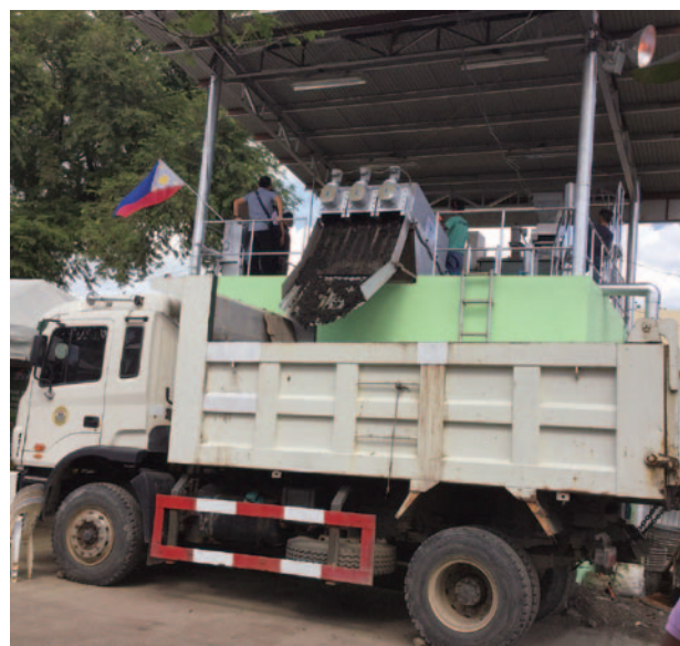
All septic tank sludge generated in the city is treated using dewatering equipment developed by AMCON INC., and after that transported by trucks. The water is treated appropriately and then released in rivers, and the solid parts can be composted. (Photo: AMCON INC.)
