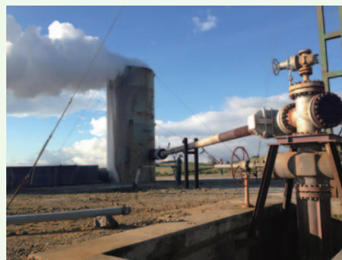
Testing steam discharge for the Guanacaste Geothermal Development Sector Loan - Las Pailas II. (Photo: JICA)
