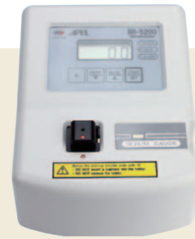
An instrument for measuring bilirubin level in blood. It is compact and lightweight. (Photo: APEL Co., Ltd.)
