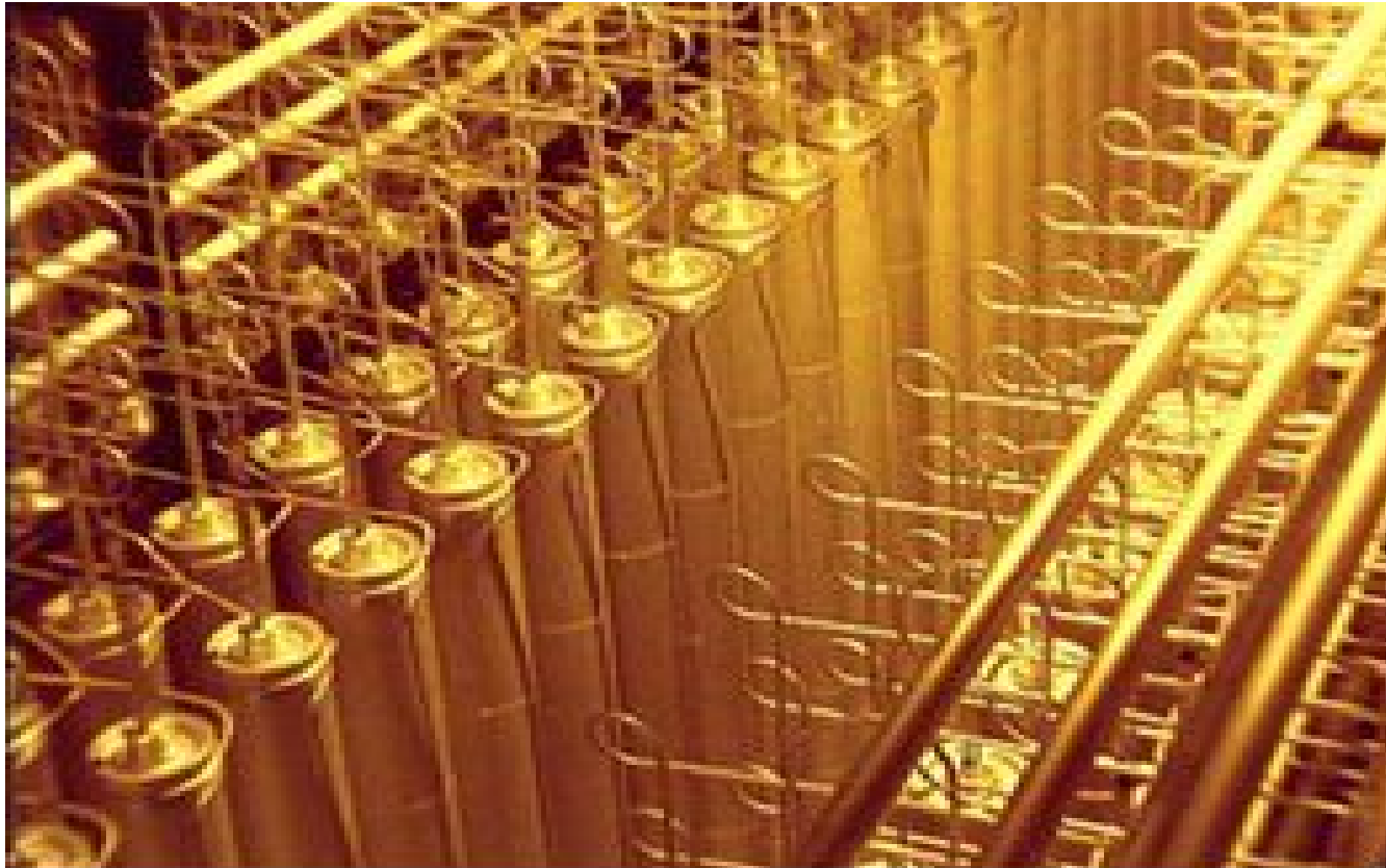
A Bank of Centrifuges at a Urenco Plant (image: Urenco)
