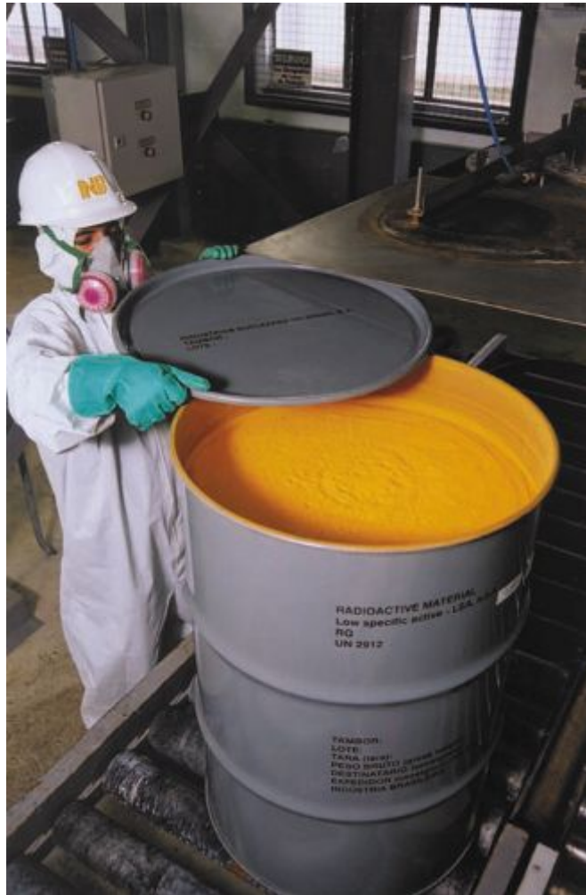
Final Product of Milling Step – 70 to 80 % Uranium
