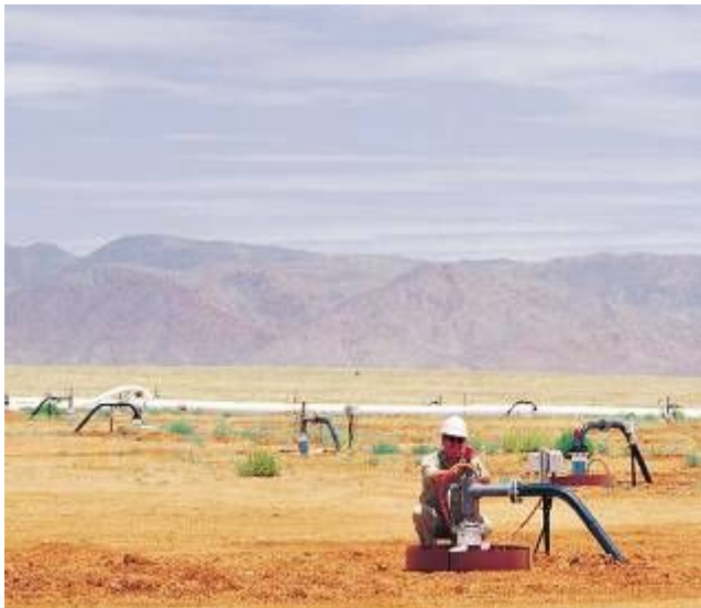
In Situ Leach Mining, Beverley, Australia (image: Heathgate)
