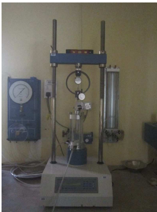
Photo -4.6 Unconsolidated Undrained Compressive Strength Test Equipment
