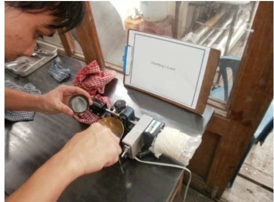
Photo -4.3 Atterberg's Limit Test
