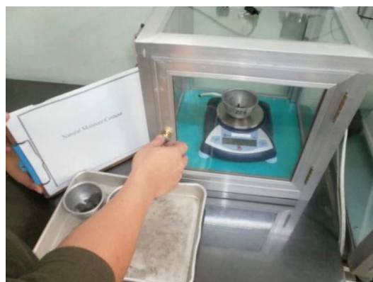
Photo -4.1 Natural Moisture Content Test
