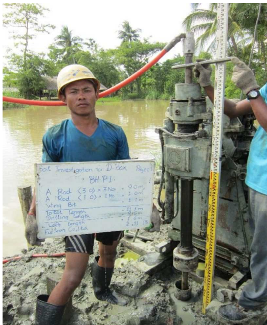
Drilling & Left Length (A)
