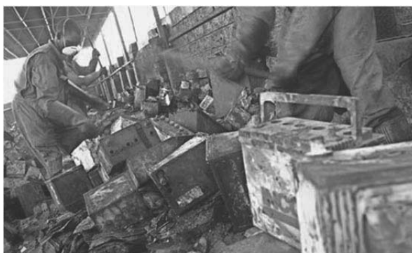
(photo) Many Kenyan youth manually extract lead plates from waste batteries 1
