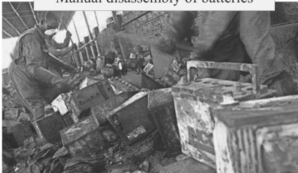
Manual disassembly of batteries
