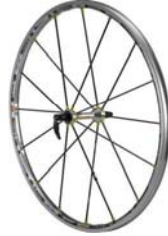
spokes of a bicycle wheel in pretension
