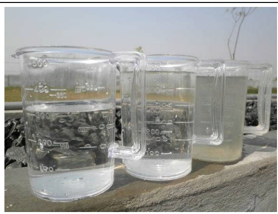
Wastewater after, during and before treated by Jarikko
