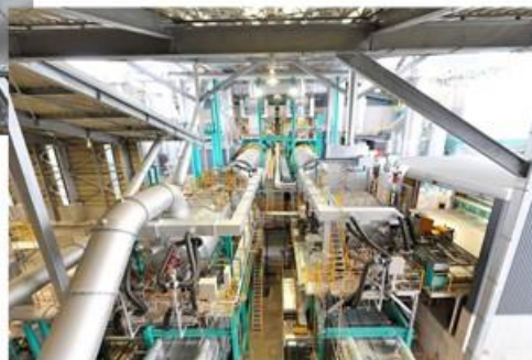
Counterflow kiln type incinerator 150×2=300t/day
