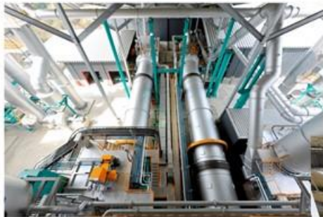
Counterflow kiln type incinerator 150×2=300t/day
