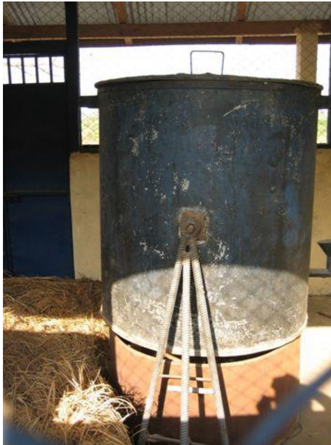
✂ Photo 9 : A steamer from the after harvest transformation chain, property of the Union of Dantilya. That transformation chain was offered by the SG 2000 Nerica pilot project : it includes a multi-tresher, a husking machine, a steamer and two drying spaces.
