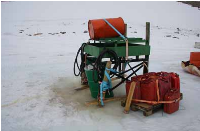
Outdoor oil dispenser (there were signs of accumulation of small amounts of oil that had leaked during oil supply)
