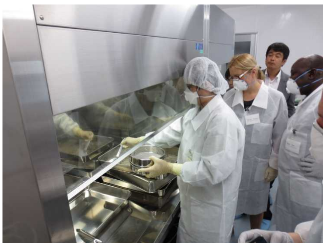
Implementation of the pre-processing of sediment required for the analysis and the resulting sets of identical samples prepared for independent analysis by each laboratory.
